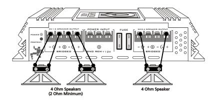
\*\*CAUTION! In the bridged mode, the amplifier must see a 4 Ohm load or higher. Any lower than 4 Ohms will cause the amplifier to overheat and possibly cause permanent damage to the amplifier!
